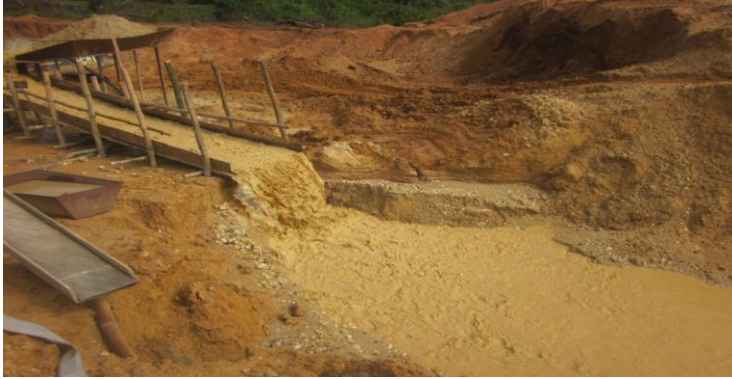
Figure 5. Disposal of Tailings from a Dredging Boat
