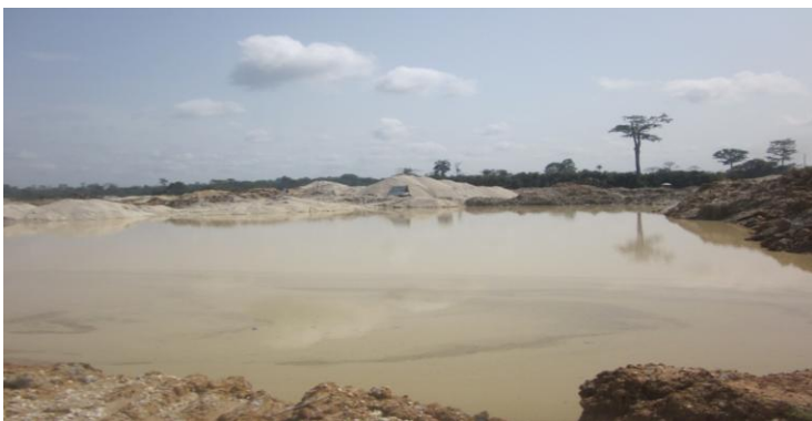
Figure 3. Pit full of Tailings Surrounded by Removed Overburden
